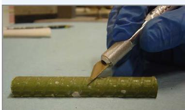
Extracted epoxy-coated bar samples underwent several tests; the dry knife adhesion test measures the adhesion of the coating to the bar.
