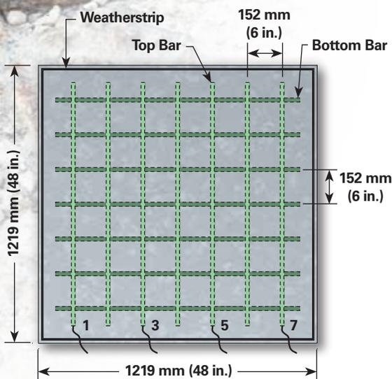
Field Test Specimen Setup —
