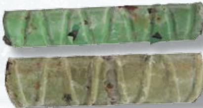
Two bars from the Ocean Isle Bridge show light corrosion: a) a horizontal No. 6 bar with a cover of 4.75 in. and bar-level chloride concentration of 0.199 wt%; b) a vertical No. 8 bar with a cover of 5.1 in. and bar-level chloride concentration of 0.183 wt%.
