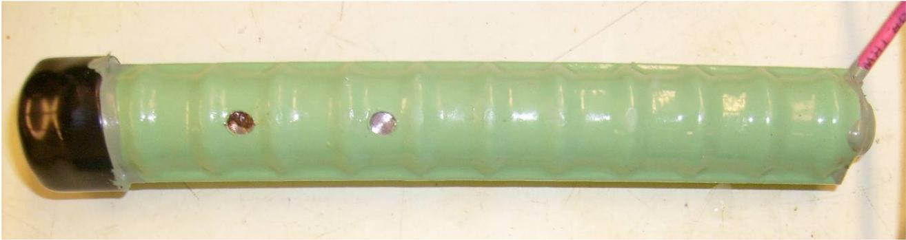
**Figure 38:** Corrosion typical of that seen on 0.83% damaged area ECR at conclusion of the test. Specimen 5, side A.
