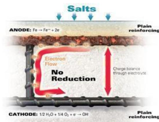
Figure 4: Corrosion of uncoated bars in concrete slab
