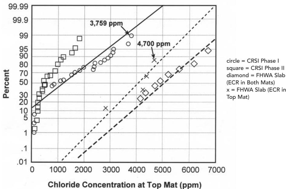
data set) was considered a representative  $C_{th}$  of epoxy-coated reinforcing bars in bridge decks with coated bars in the top mat only. However, it was not possible, based on the data available, to derive a statistically significant value of  $C_{th}$  for epoxy-coat-
