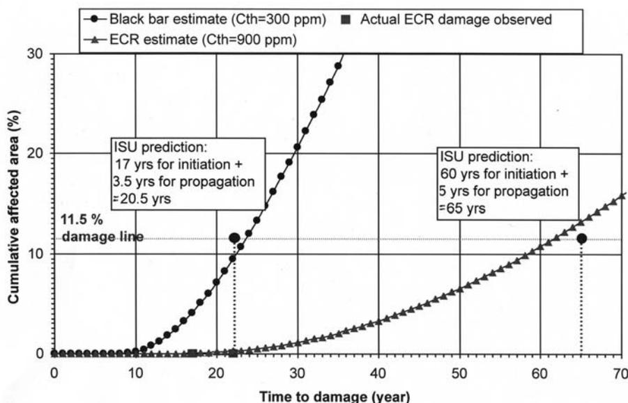
time-to-damage curves were also developed assuming that the bridge decks were reinforced with uncoated reinforcing bars, epoxy-coated reinforcing bars in the top mat only, or epoxy-coated reinforcing bars in both mats.
