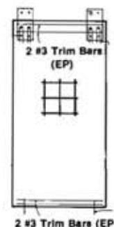
Diagram shows locations of No. 3 epoxy-coated rebars at perimeter of panels. No. 4 uncoated rebars are on 12" centers in the rest of the panels.
