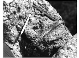
A field exposure test to evaluate the performance of marine reinforced concrete structures was recently conducted by the Department of the Navy. The test findings were presented at The International Conference on Corrosion and Corrosion Protection of Steel in Concrete at the University of Sheffield, England during July 1994. Prepared by Douglas Burke, at the National Facilities Engineering Service Center (NFESC) the report, "Performance of Epoxy-Coated
