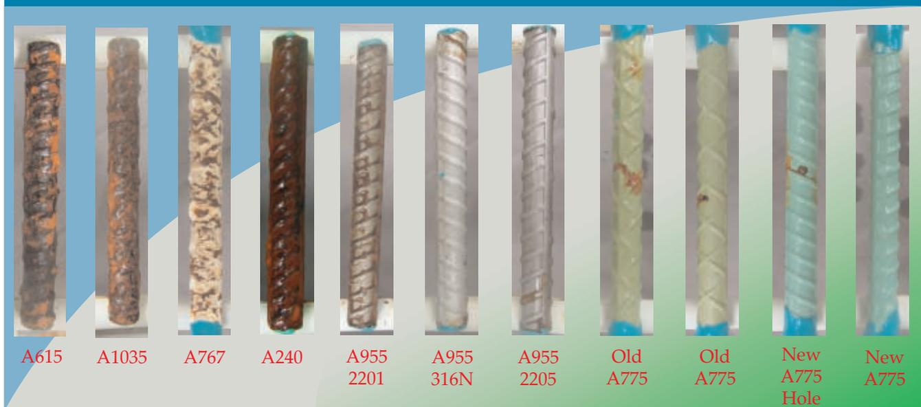
All bars tested 'as received' except the epoxy-coated bar indicated had a 1/16 inch hole drilled
