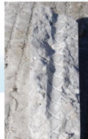
Concrete core sample with smooth, unstained rebar impression
