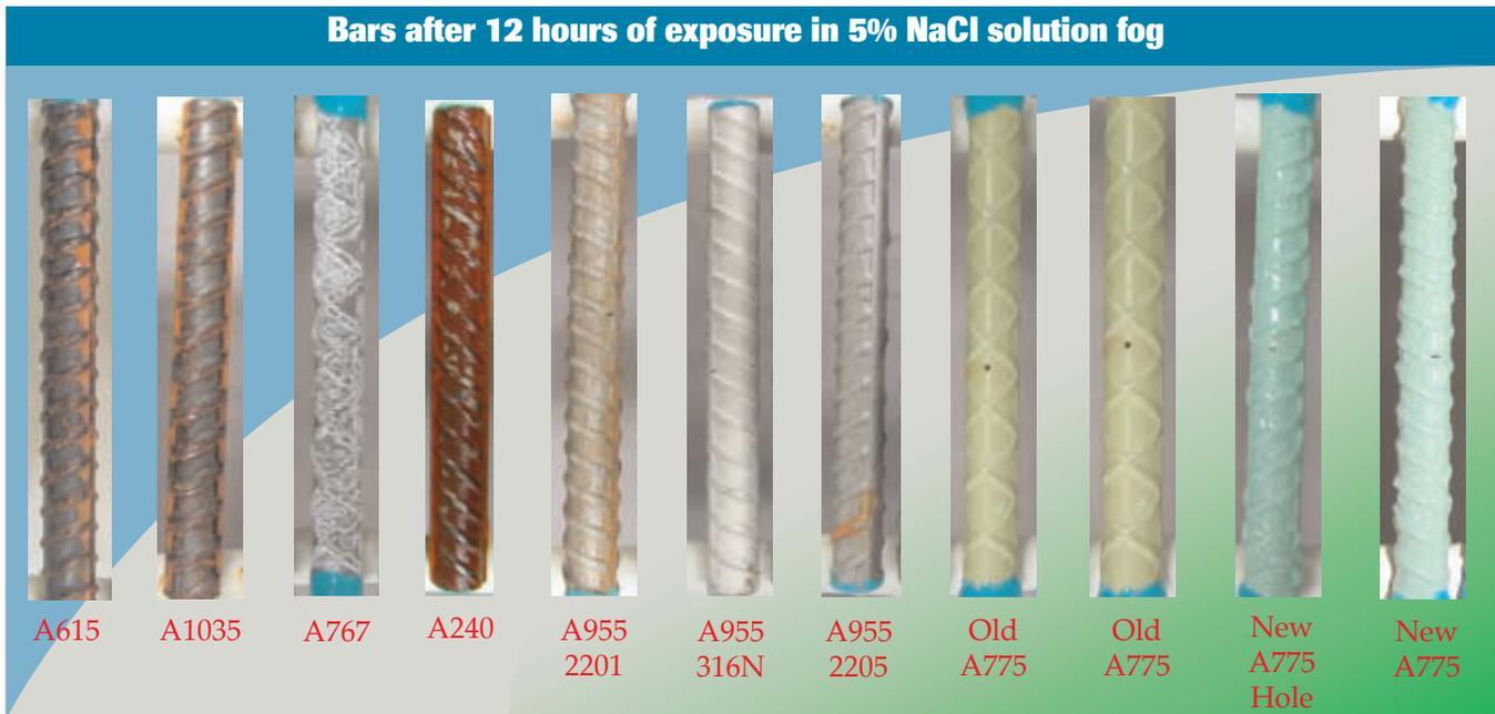
All bars tested 'as received' except the epoxy-coated bar indicated had a 1/16 inch hole drilled
